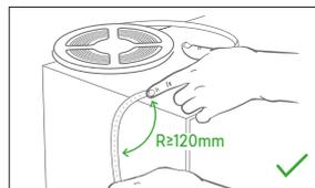
During normal service, once need a turning, must hold the curve of LED strip with its front side up and back side down.
