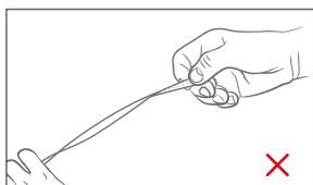
The LED strip can not be distorted during normal service.
